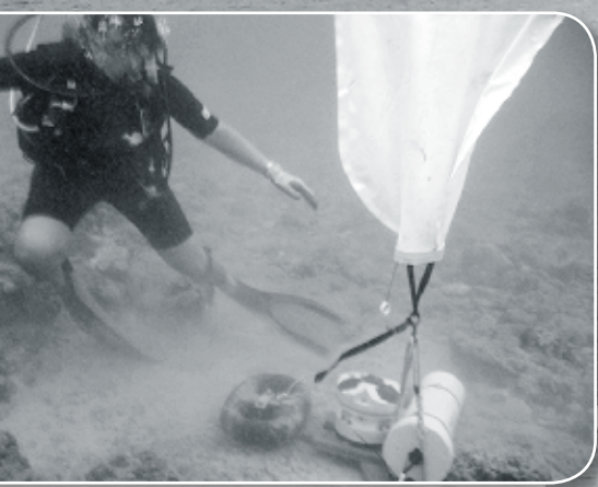
Diver with an Acoustic Wave and Current (AWAC) profiler on the bottom of Hanauma Bay.
